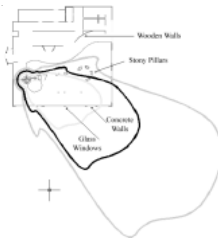
Figure 1: Coverage prediction of the antenna in the Parmer restaurant. Various partition types are described using arrows and texts.
